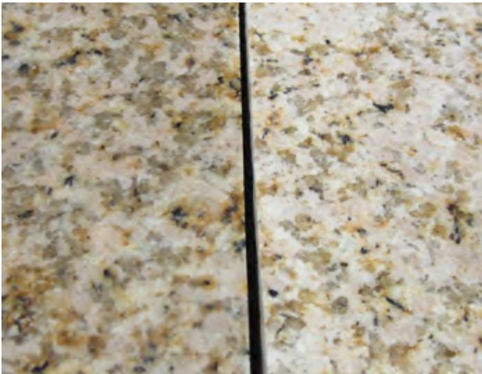
The picture above indicates how the untreated sample became darker after 24 hours of immersion into water, while the SurfaPore M treated sample remained unchanged.
