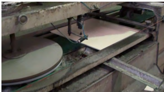
Figure 1 - Application of T51 on polished tiles at Revigrês
